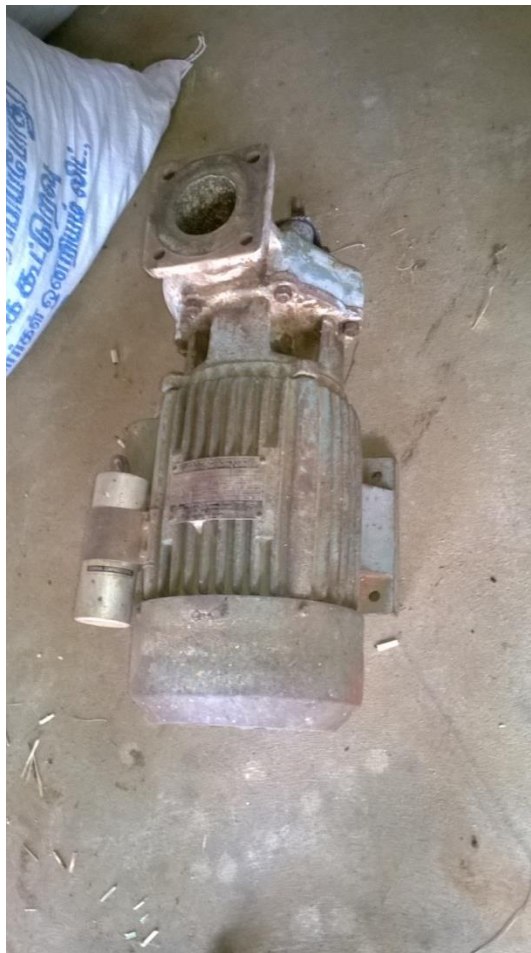
C.R.I. ACM 21 - 1 Phase, 230 V, Hz - Centrifugal Monoblock Pumpset, 2840 rpm - 13 Years old, still running without any trouble.
